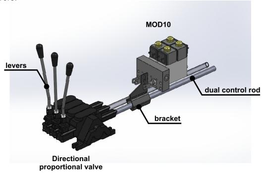
MOD10 pushes/pulls the brackets and causes the movement of the spool through the dual control rods.
