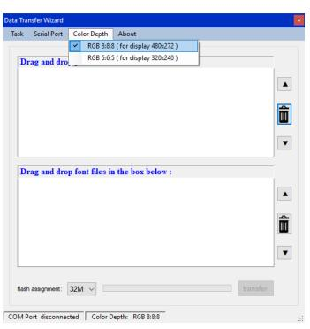
Select the correct COM port via "Serial Port" and connect to the  $\mu$ C via the "connect" button. The text "connected" with a green background should then appear in the bottom left-hand corner. Now select the appropriate display type via "Colour Depth":
