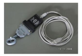
The NBB programmes communicate with the microcontroller via the serial interface. As most modern computers no longer have this interface, a converter is required. The NBB USB-Serial Adapter is used for this purpose. This makes it possible to simulate a serial connection to the microcontroller and to programme it.
